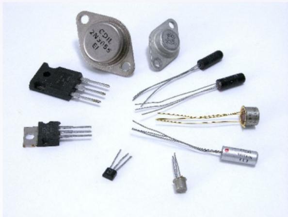
2nd Generation: Semiconductor Devices, Diode and single Transistor
